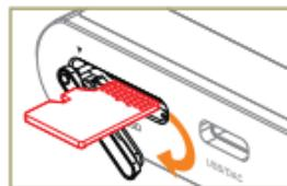
3. Twist the cover out of the way to access the Micro SD card.
