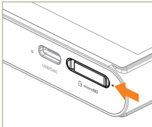
1. Lift the card cover by pulling on the marked edge of the card cover.
